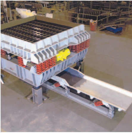
Ladle Shakeout with Slag Takeaway Conveyor.
