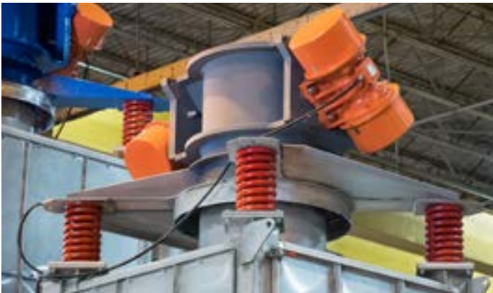
Steel Heat Shield Protects the Spiral Motors
